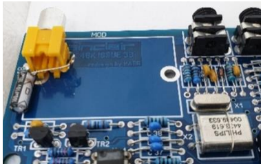
Direct installation of the video jack
